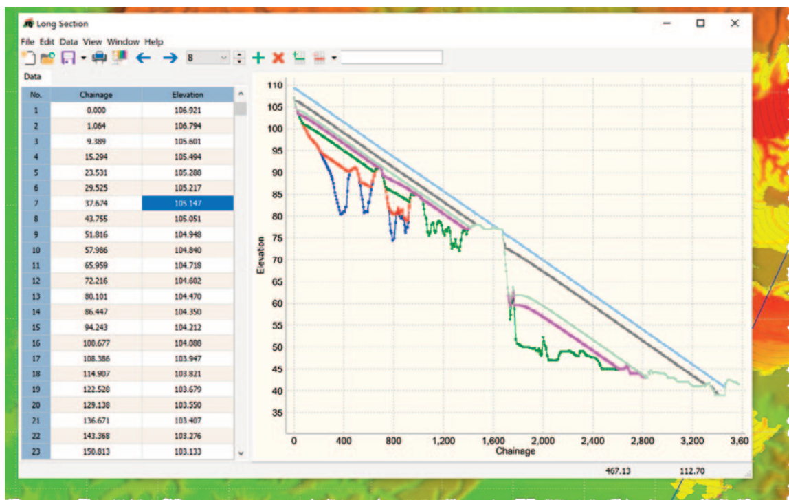
Longitudinal Sections along Several Raise Surfaces
