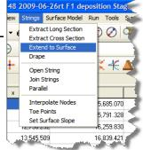
If neither the start or end String points is on the surface you will be prompted to indicate a String side to extend; if one of the String points is already at the surface elevation the other end string point will be automatically extended to the surface.
